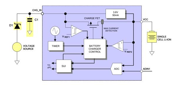
Figure 5.7-1 Typical application for pulse charging a battery
